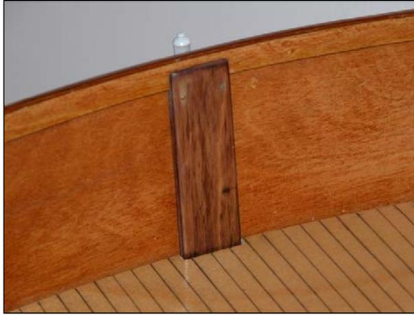
**Fig 21** Transom wiring cover in position
