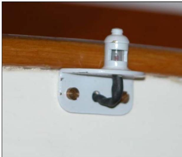
**Fig 14** Stern Light mounting using a Brass Bracket
