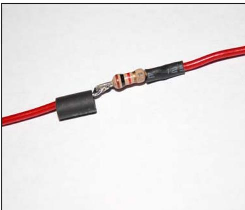
**Fig 33** Resistor in Positive Lead
